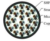
SHF2 Sheath Stranded Copper Conductor Mica Tape + HFEPR Insulation Copper/Polyester Tape + Drain Wire
